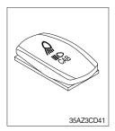
(1) This switch use to operates the switch illumination lamp and work light by two step.
