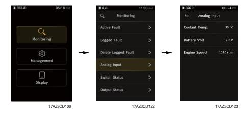
The machine status such as the engine speed, coolant temperature, battery voltage can be checked by this menu.
